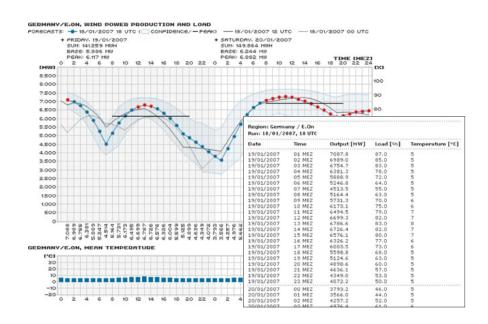
To assure a constantly high accuracy, EuroWind applies multiple numerical weather models for the calculation of the individual power output of each wind engine and adds them together for optional areas, such as control areas, provinces or wind parks.
